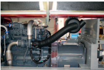
Air supply from the air filter to the engine
